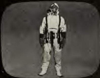
SHALLOW-WATER lightweight dress for cold-water quick dives for repair, uses wide-vision mask. Ship feeds air.
